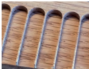
Chip-free dovetailing using a LEUCO p-System shank-type grooving cutter
