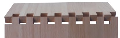
Chip-free dovetailing using a LEUCO p-System shank-type grooving cutter
